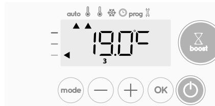
In case of programmed Boost, the Boost activation will take precedence over others orders received except when the standby (stop) order is present on the pilot wire, the device will switch off and the Boost will be not activated.
