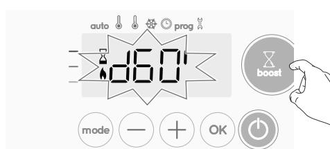
During the first minute, you can modify the Boost duration from 0 to the maximal authorised duration of the Boost, such as defined during the advanced settings (see page 13 for more details) by intervals of 5 minutes (or more quickly by push superior to 2 seconds) by pressing and . This modification will be saved and effective for the next Boost.
