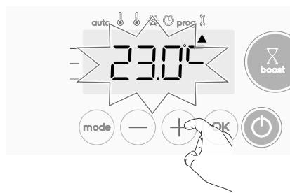
To validate, save the new value and exit the mode, press **OK**. To exit the Expert settings, press **mode** 3 times.
