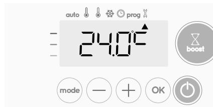
Decrease the temperature measured by the ambient temperature sensor by 2°C by pressing (−).
