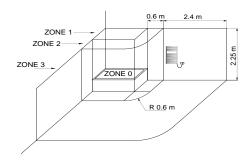
The national rules on installing electrical equipment in the bathroom must be scrupulously respected. The electric radiators must be always installed outside zone 1 and 2. In particular the electric switch and control elements must be mandatorily located in zone 3, in order that no electrical control center is accessible to anyone using the shower or bath.
