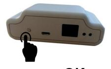
2) Press at the radiator the button MODE/OK for 3 sec. to link.
